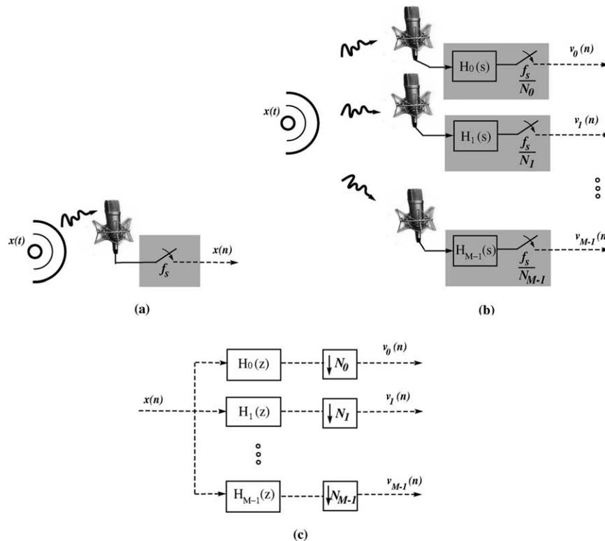
Fig. 1. A direct high-sampling-rate measurement (a) is emulated by a collection of low-sampling-rate measurements (b). The relation between the high-rate signal  $x(n)$  (which is the object of measurement but not available) and the available low-rate measurements  $v_i(n)$  can be modelled using a multi-rate filter bank as shown in (c).
