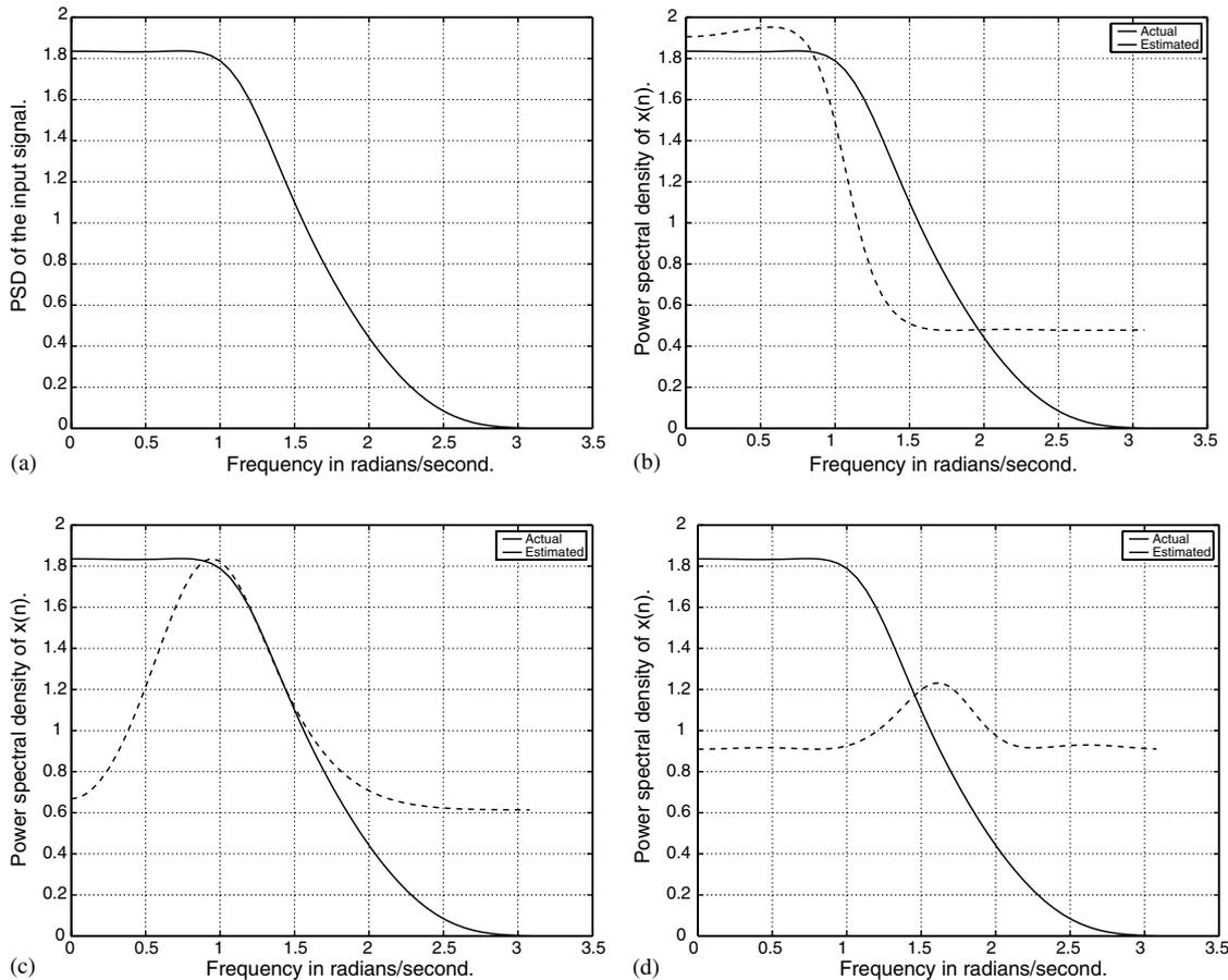
Fig. 6. (a) Actual power spectral density of the non-observable reference signal  $x(n)$ . The plots (b)–(d) show the PSD estimates  $\tilde{P}_x^{(i;4)}(e^{j\omega})$  obtained using N-MEIE for individual channels of the 3-channel low-resolution measurement system. The plot in (b) shows the estimate obtained using Channel 1; (c) shows the result obtained using Channel 2 and (d) shows the result obtained using Channel 3.
