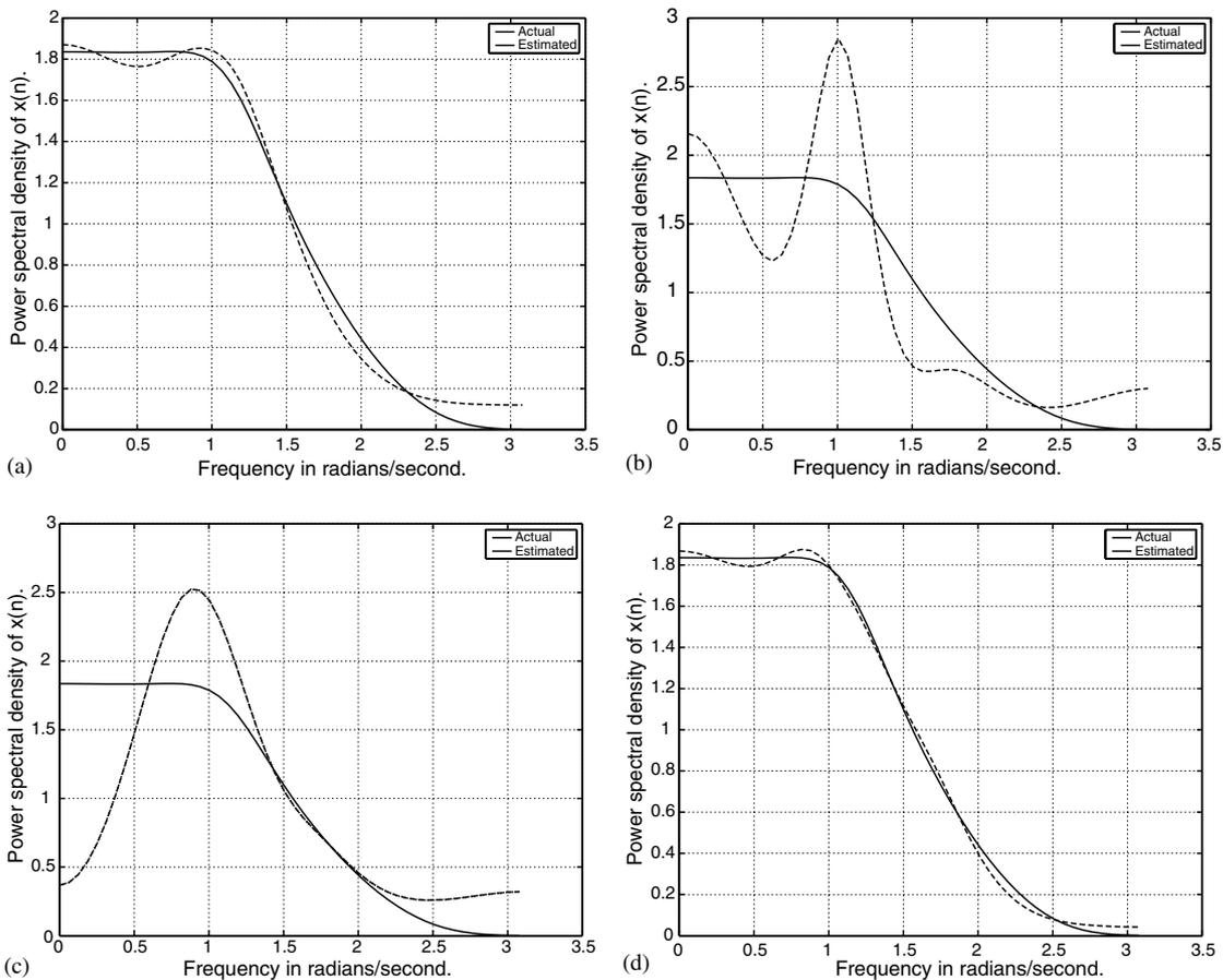
Fig. 7. Power spectral densities  $P_x^{(i;4)}(e^{j\omega})$  estimated by N-MEIE by combining the low-resolution data provided by individual channels of the measurement system: (a) Channels 1 and 2, (b) Channels 1 and 3, (c) Channels 2 and 3 and (d) Channels 1, 2 and 3. Note that the scale in plots (b) and (c) has changed to accommodate the overshoots that exist in the estimated PSDs.
